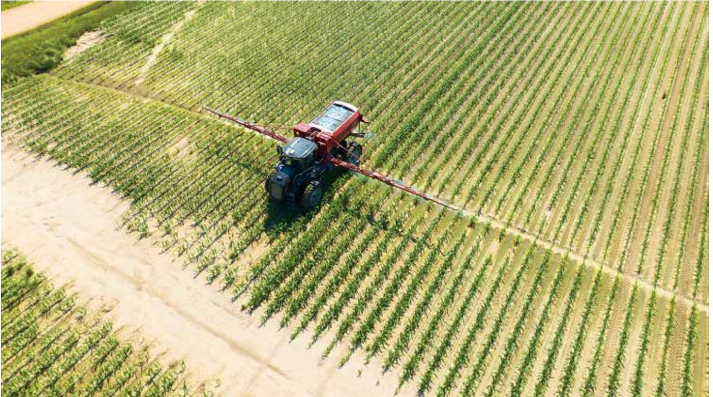
When we started, we would manually drive the machine through the field, laying soap foam as a guidance tool. Today we use auto-steer and satellite GPS to know where we are in the field. We can variable-rate apply fertilizers – The consultants do grid sampling and write an actual prescription for the fertilizer so each acre gets just the amount of fertilizer it needs. This saves the farmer money and it helps in conservation by not over-applying fertilizers.”
